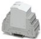
Plug-in device protection, according to type 3/class III, for 3-phase power supply networks with separate N and PE (5-conductor system: L1, L2, L3, N, PE), with integrated surge-proof fuse and remote indication contact.
